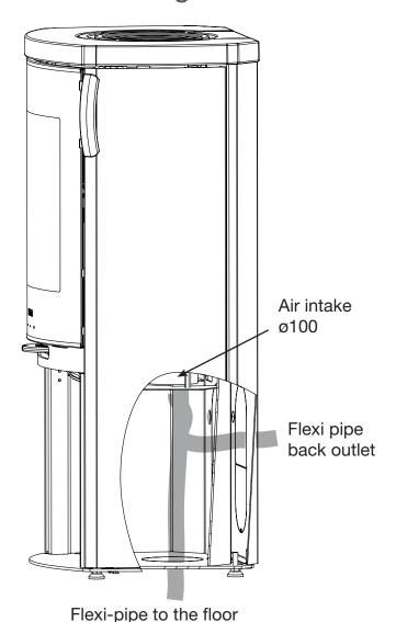
When installing external air supply, connect the air intake to the direct air pipe using flexi-pipe, both from the floor or behind the stove.
