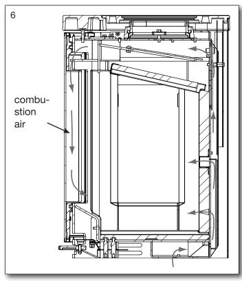
The chimney height and diameter, as well as the temperature difference between the flue gas and outside temperature generates the chimney draft. Chimney insulation is therefore important as new efficient stoves create lower flue temperatures. Wind and weather conditions also influence draft, in some cases it may be disadvantageous wind direction, combined with the position of the chimney can cause negative draft (it blows through the chimney), causing smoke escape from the stove.
