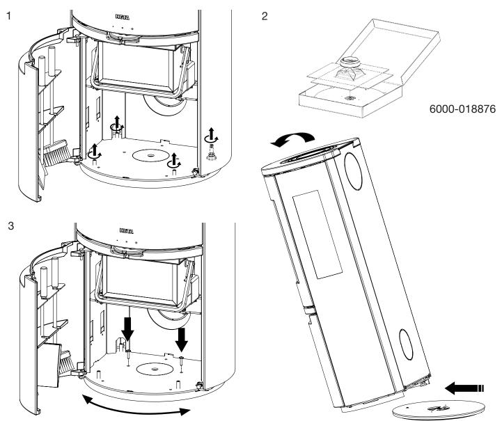
External fresh air mounting on rotating base for Scan-Line 900
